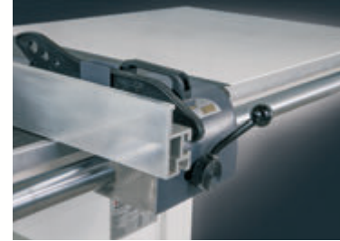
Kolay Siper Ayarı Quick Adjustment of Rip Fence
